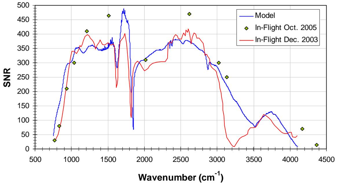
Figure 3: Comparison of SNR model prediction (blue) and in-flight measurements in 2003 (red) when there was ice before deicing and in 2005 (green).
