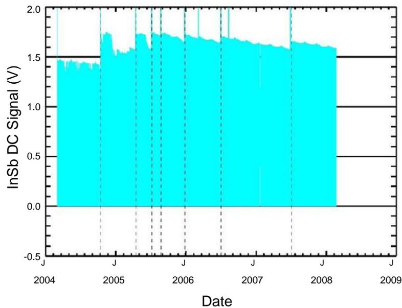
Figure 14: Evolution of the DC signal level of the InSb detector with time
