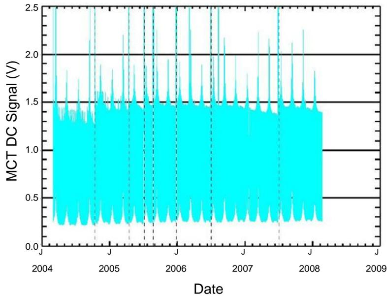
Figure 13: Evolution of the DC signal level of the MCT detector with time
