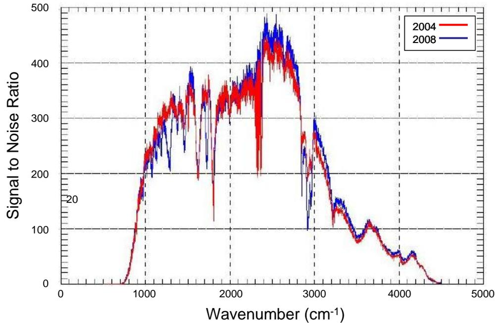
Figure 5: On-orbit SNR comparison of 2004 (blue) and 2008 (red). Each curve was built with exoatmospheric measurements during five occultations at beta angle near  $0^\circ$
