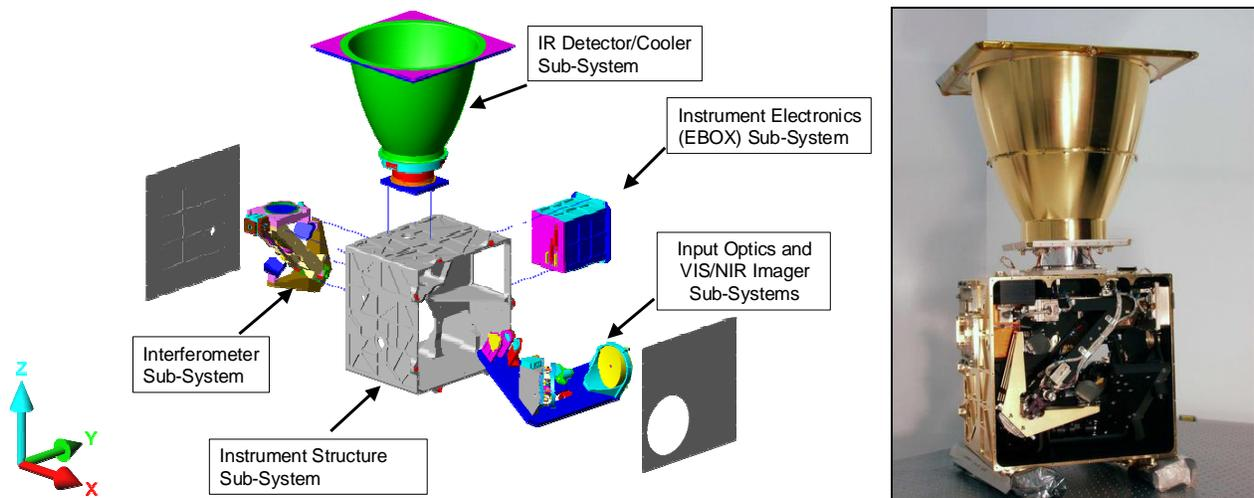
Figure 2: ACE-FTS architecture (left) and picture of the Flight Model (right)
